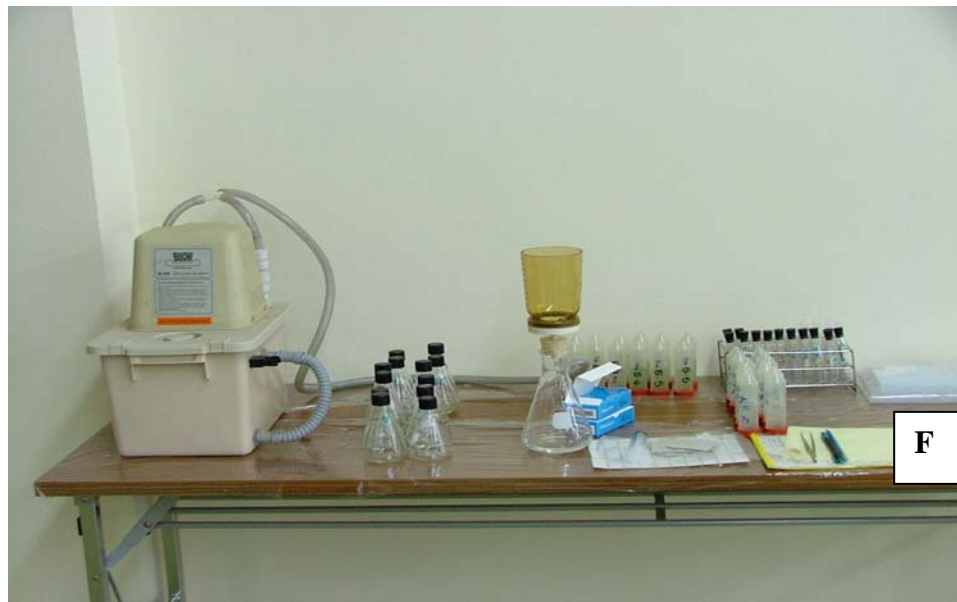
Figure 1C (Continued). E. Total Reflectance (ATR) accessory, F. Vacuum filtration with glass fiber filter
