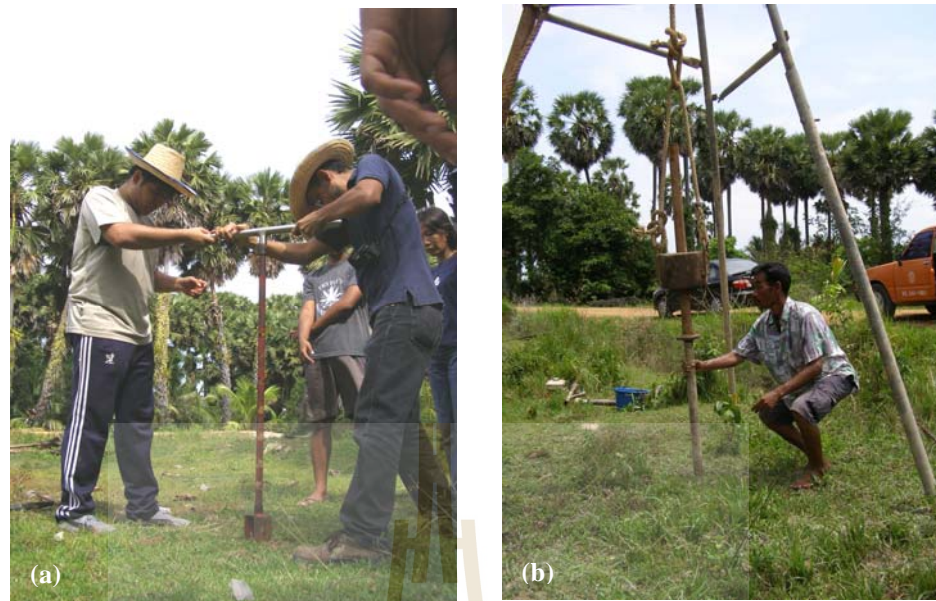
Fig. 3.3 Photographs of core sampling for core no. SUT-1: (a) coring by hand auger; (b) coring by piston corer. (photographed by Pikun Sittiprasertkun)
