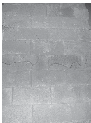
a) Crushing lines on the compression surface
