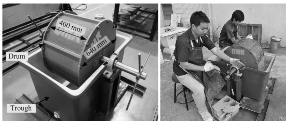
Figure 2. Drum constructed for large-scale slake durability test.
