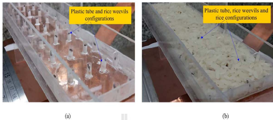
Fig. 19. Constructions of dielectric load configurations, (a) the rice weevils are placed in the center of plastic tube with diameter of 4.8 mm and arrayed of 5 \times 9 points (b) The dielectric material of rice is dispersed around the plastic tube.
