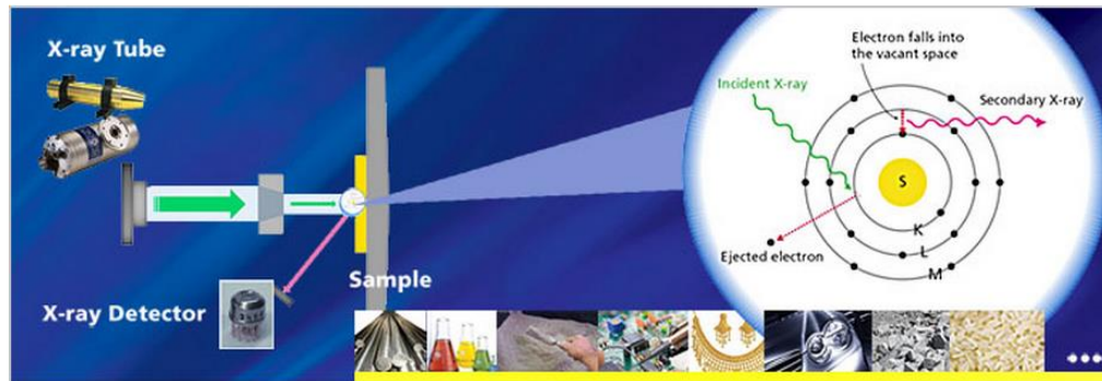
Figure 2.4 A schematic of the work processing of XRF analyzer (Oxford-Instruments.com, 2015).
