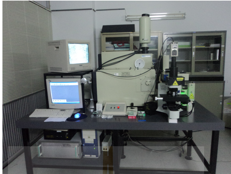
(a) JOBIN YVON HORIBAT64000 Raman spectroscopy system at Chiang Mai University.
