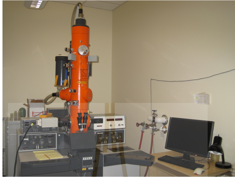
Figure 3.8 Zeiss CEM 902 TEM (University of Phuket Sound)
