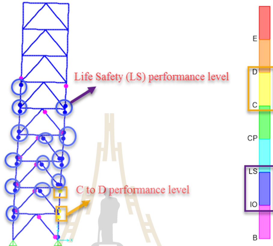
Figure 4.8 Plastic hinges of the braced steel frame
