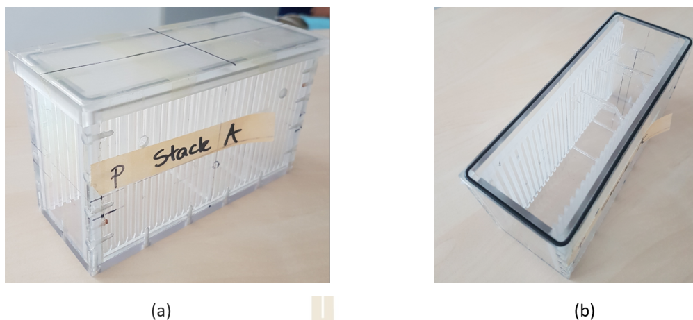
Figure 3.2 Stack phantom consists of PMMA box and polystyrene slides: a) outside part and b) inside part where slides are arranged.
