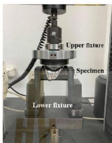
Fig. 4. The universal testing machine for experiment of contact stress distribution using Fuji film technique
