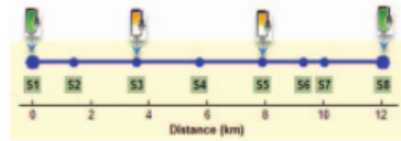
Fig. 13. Option III: Charging points installed at terminal stations and one of the intermediate stations
