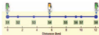
Fig. 10. Option II: Charging points installed at terminal stations and one of the intermediate stations
