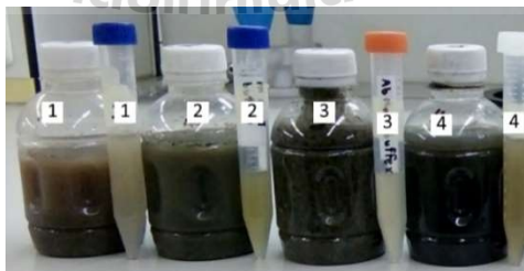
Figure 4.1 Soil sample and washed by 0.85% NaCl and filtered in centrifuge tube 15 ml. 1) slaughterhouse, 2) pigsty, 3) pig manure wastewater treatment plant, and 4) biogas generator.
