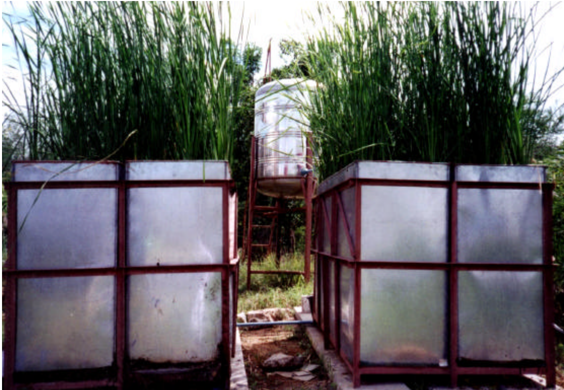
Figure 3.4 The four reactors of constructed wetlands
