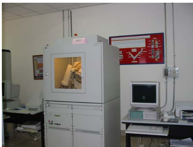
Figure 3.9 Bruker, model D5005 X-ray diffractometer with Ni-filtered Cu K_{\alpha} radiation.
