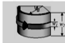
Fig.3 The structure of a curved strip dipole without reflector plane.
