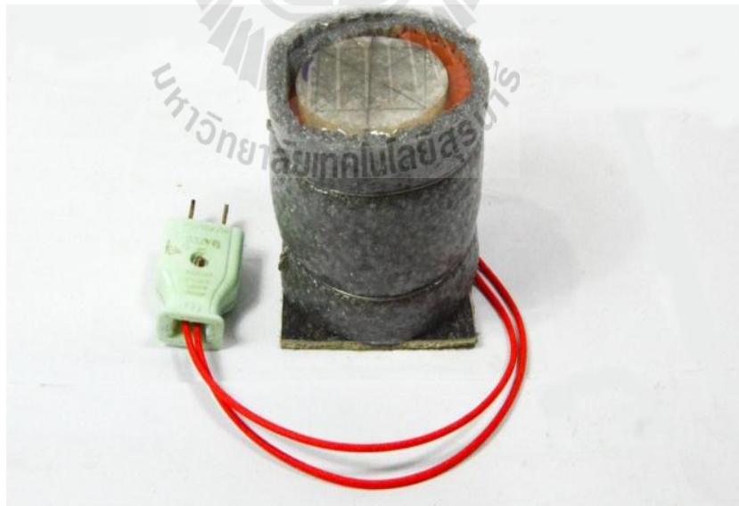
Figure 4.3 A salt specimen is wrapped with heating tape, foil and isolator before testing to maintain constant during the test.
