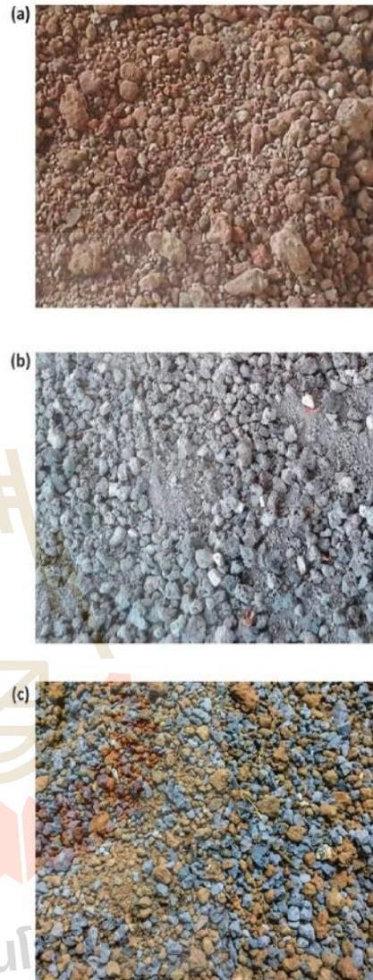
Fig. 1. (a) Lateritic Soil (CS) (b) Crushed slag and (c) Lateritic soil/CS blends.
