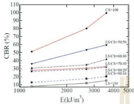
Fig. 4. Soaked CBR versus compaction energy relationship of lateritic soil/CS blends.
