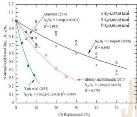
Fig. 7. Normalized swelling versus compaction energy relationship of lateritic soil/CS blends.
