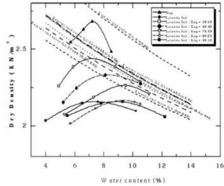
Fig. 3. Dry density versus moisture content relationship of lateritic soil/CS blends.
