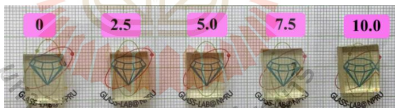
Figure 6.1 Photograph of glass samples with varying Gd 2 O 3 concentrations in 25Li 2 O-5Al 2 O 3 -YGd 2 O 3 -(69.0-Y)B 2 O 3 -1.0Eu 2 O 3 (LAEUB) glasses.
