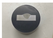
Figure 5. Metallographic hot mounting Sample
